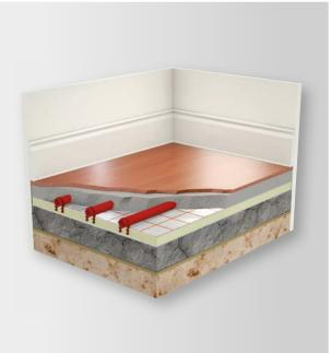
It is supplied with 25 or 50mm insulation with a webbing foil bonded to the surface. This foil acts as a protective layer, but also helps to assist the positioning of the pipework with a handy 50mm grid marked on. The pipe is then positioned in place using our exclusive Tackernails and Tackertool. It is also very flexible allowing both spiral and serpentine laying patterns.
