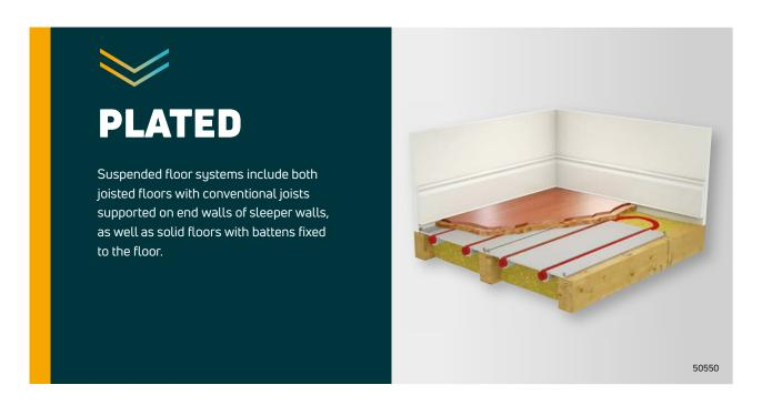
The underfloor heating system consists of aluminium diffusion plates fitted between joists or battens. These are grooved to accept the underfloor heating pipework. The aluminium plate is used for its excellent thermal conduction as well as its low weight. It is suitable for 16 and 17mm pipework.
