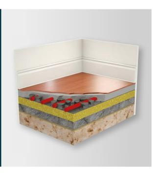
It excludes the 11mm polystyrene insulation that comes with Preformed Plate and is a cost-effective alternative. It is more streamlined and therefore ideal for areas where space is critical. It is a castellated fixing system with raised burls that are designed to firmly grip the MYSON FLOORTEC underfloor heating pipe. The pipe is fixed easily into the desired pattern by lightly pressing with your foot.
