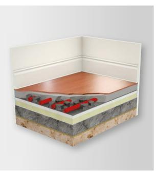
It is a castellated fixing system that comprises of an expanded 11mm polystyrene insulation base with raised burls that are designed to firmly grip the MYSON FLOORTEC underfloor heating pipe. The pipe is fixed easily into the desired pattern by lightly pressing with your foot.
